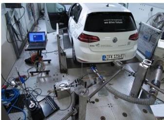
Emission measurement at a hybrid vehicle
