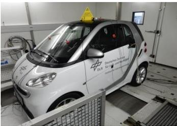
Measuring the electrical range of an electric car
