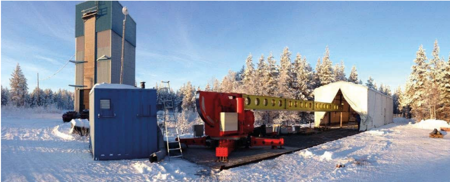
Fig. 4-3 MAN 2 Mobile Launcher with movable tent for preparation phase
