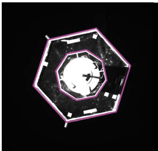
Fig. 2-1 Exemplary image of a mono camera taken at the DLR's EPOS 2.0 facility and the result of the pose estimation (visualised by model edges projected back to the image).
