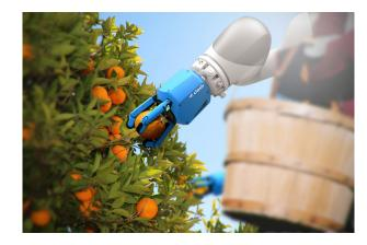
When grasping an orange, for instance, the fingers can be made soft so that they can adapt to the object shape therefore increasing the number of contact points with the object. Afterwards, the fingers increase their stiffness without increasing the applied forces, in order to safely lift the object without damaging it. This mechanism is inspired by human hands, where cocontraction of antagonistic pairs of muscles leads to an increase of hand stiffness.
