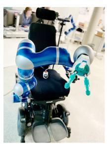
The hand design and its variable stiffness can be exploited for grasping from highly fragile objects to rigid and heavy ones (up to 2kg), using both fingertip and power grasps, and achieving success rates of up to 95% in continuous pick and place actions. The hand is further equipped with several sensors, such as tactile sensors at the palm and force and position sensors in the fingers. Another distance sensor in the palm can measure the distance to an object.
