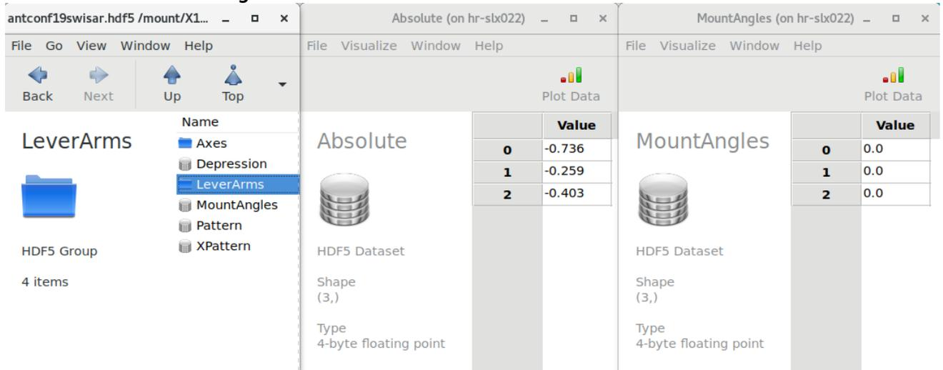
The lever-arm of each antenna corresponds to the 3D displacement, in the instrument rest frame, from the reference point of the navigation data to the antenna phase center. The lever-arm that is relevant to SAR processing is held in the "Absolute" data set of the "LeverArms" sub-group. The lever-arm axes denote offsets in flight direction, towards the left and upwards, respectively. Lever-arms are given in *m*.
