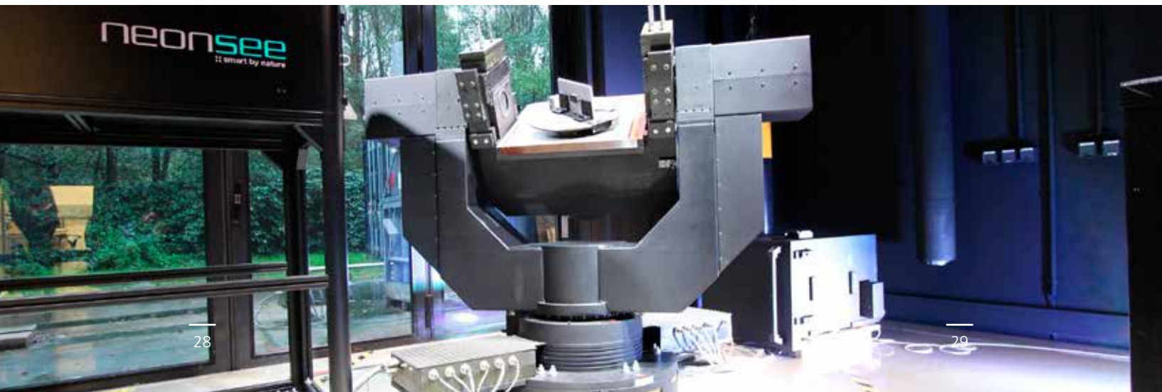
STARS Testbed with Sun Simulator and Rotation Table
