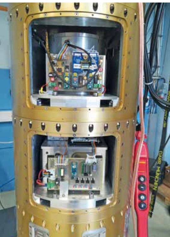
The sounding rocket modules for MemEx (top) and CellFix (bottom) integrated into the rocket shell structure.
