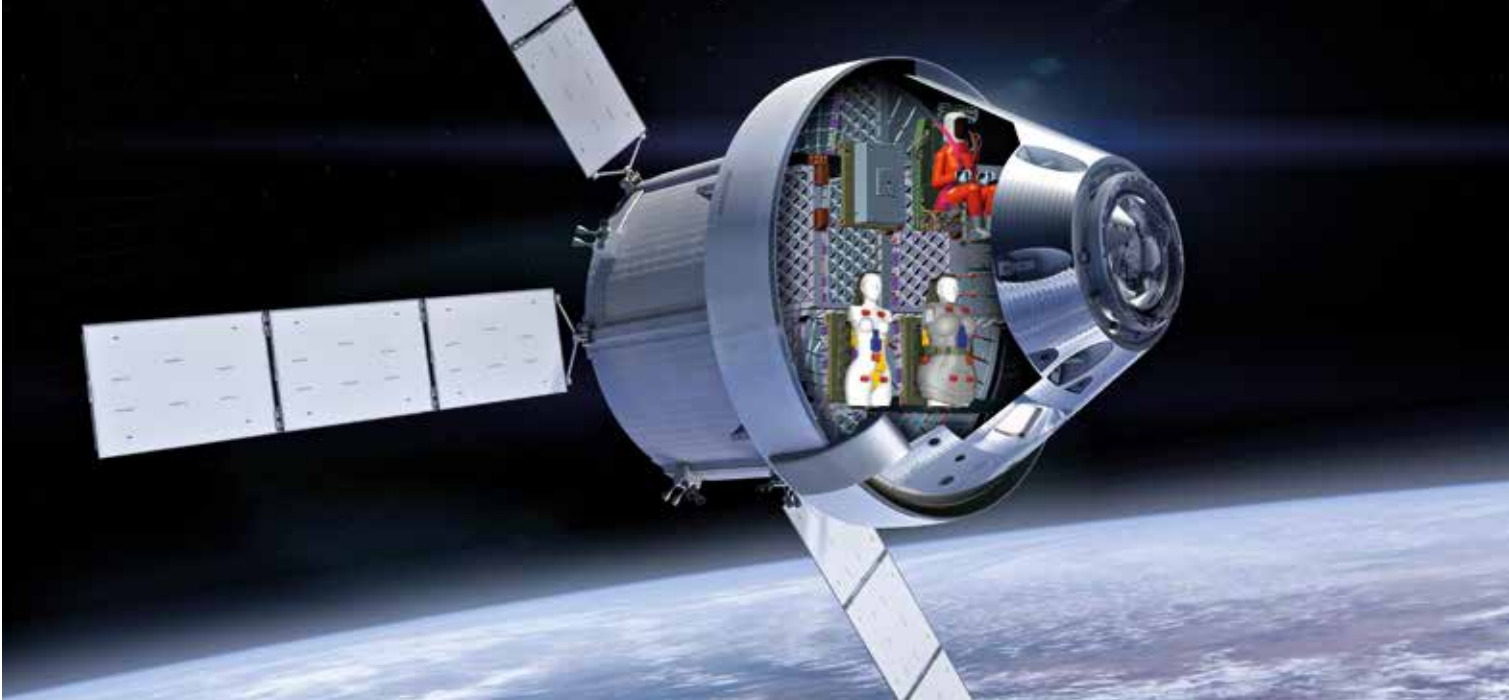
The MARE experiment with HELGA and ZOHAR in the NASA Orion spacecraft for the Artemis I mission.
