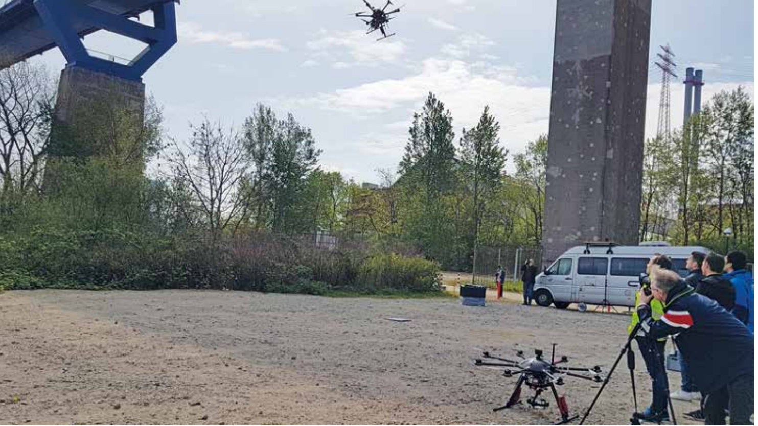
Drone flight for bridge inspection
