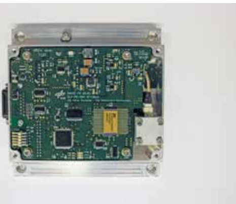
The RAMIS radiation detector flying on the DLR Eu:CROPIS mission
