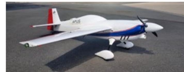
APUS, a research aircraft with a powerful engine for towing
