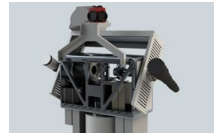
Model of the pan/tilt platform for the identification and precise route tracking of drones
