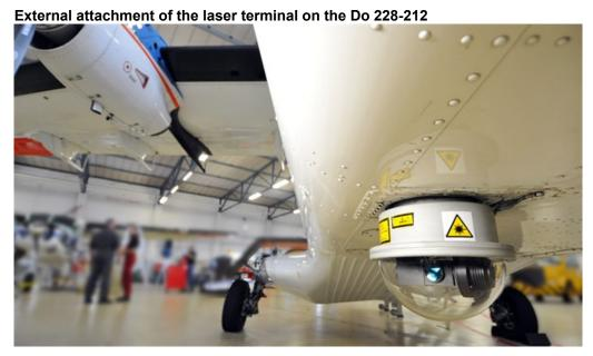
The external part of the laser terminal is attached to the fuselage of the DLR Do 228-212 research aircraft.
