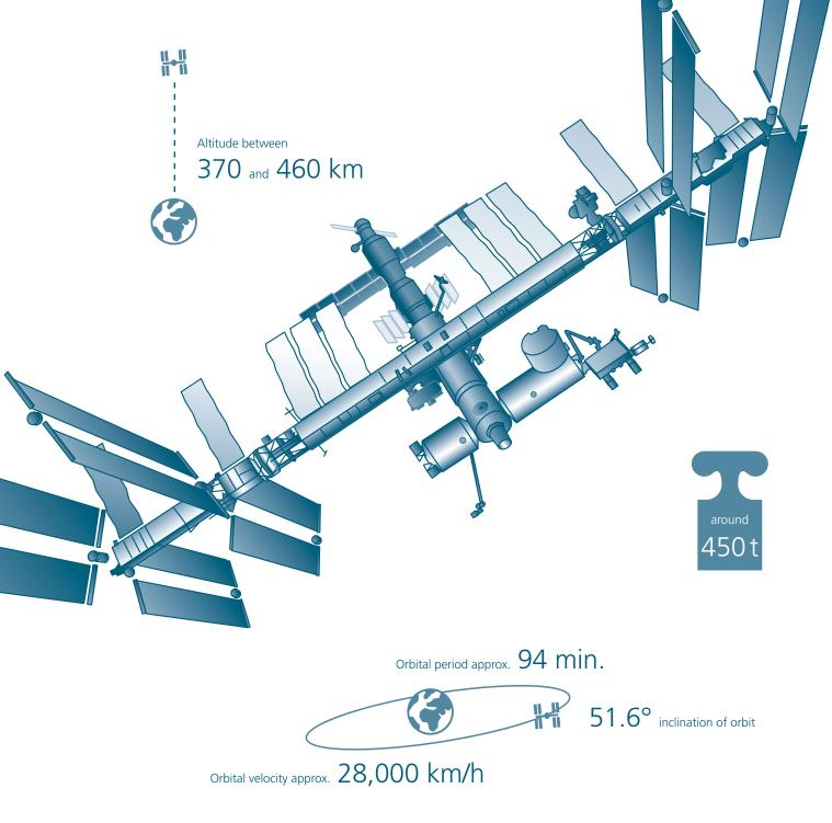
horizons – International Space Station ISS Facts and figures The ISS is humanity's largest technology projec Germany finances 41 per cent of the European contribution to utilisation of the ISS. 262,400 solar cells extend over 2500 m and provide the astronauts on the ISS with as much electrical power as is required by 40 homes. 110 kW The ISS was assembled in 32 stages over a period of 12 years. The components were flown into space via 36 Space Shuttle and five Russian launches. 199
