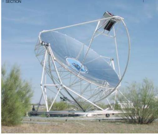
Figure 6 The EURO-DISH parabolic dish concentrator with a Stirling motorgenerator in the focal point at the CIEMAT solarthermal test centre Plataforma Solar de Almeria, Spain (Source: SBP)
