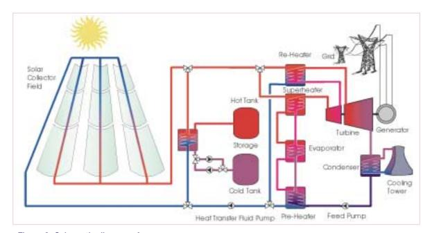
Figure 2 Schematic diagram of a steam cycle power plant with a parabolic trough collector and a thermal energy storage (Source: DLR)
