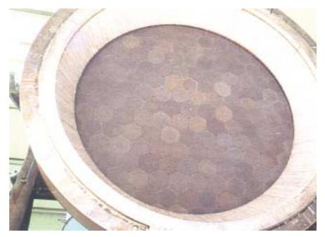
Figure 8 Volumetric receiver (Source: DLR)
