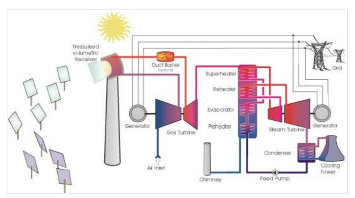
Figure 10 Schematic of a combined cycle system powered by a volumetric central receiver using pressurised air as heat transfer fluid (Source: DLR) grid-connected dispatchable markets and remote or modular distributed markets. Parabolic troughs, central receivers and parabolic dishes will be installed for solar/fossil hybrid and solar-only power plant operation. In parallel, decentralised process heat for industrial applications will be provided by low-cost concentrated collectors.
