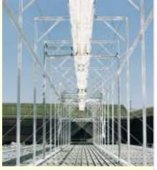
Linear Fresnel collector at the Solarmundo test facility in Liege, Belguim
