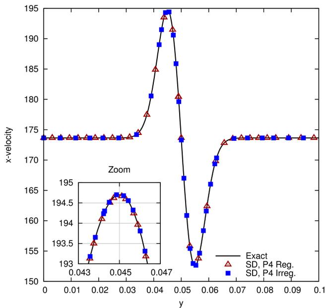
Figure 5: Case  $M = 0.5$ : x-velocity profile on regular and irregular grids
