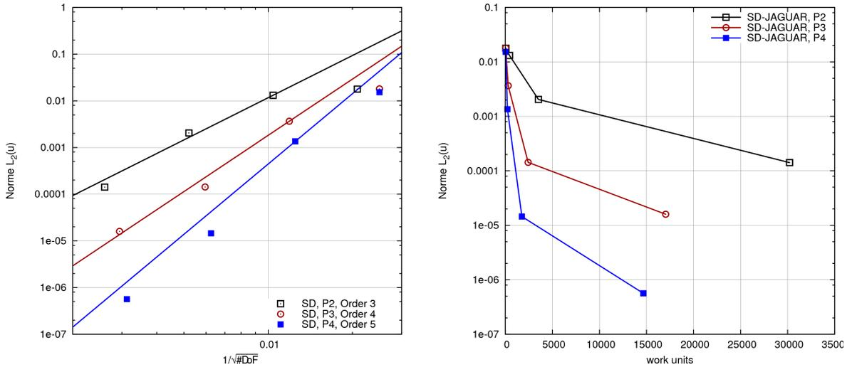
Figure 3: Case  $M = 0.05$ : grid convergence on the x-velocity profile after 50 periods
