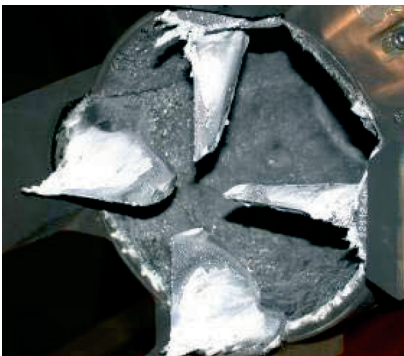
C/C-SiC jet vanes before (above) and after (below) firing in a suitable bench.
