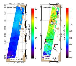
Meteo-marine parameters processed from TerraSAR-X data acquired over the German Bight on 07.04.2015 at 05:50 UTC. The acquisition consists of four individual images and covers an area of 30 km × 250 km with resolution of 1.2 m pixel size. Significant wave height  $H_s$  and surface wind speed  $U_{10}$  are processed with 3 km × 3 km posting.
