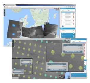
Screenshot of the SAR wind and wave product on Web Mapping Server at Ground Station Neustrelitz. The sea state and wind estimation algorithms are implemented into the NRT server chain. The maritime environment: wind (arrows) and sea state (circles) are combined in layers. The demonstrator runs daily for Sentinel-1 IW in southern North Sea and western Baltic Sea.
