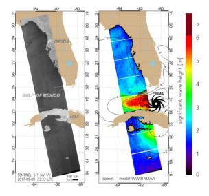
Significant wave height  $H_s$  estimated from a Sentinel-1 scene that covers approximately an area of 250 km × 1500 km, consisting of eight individual images. The acquisition was taken over Cuba and Florida on 09.09.2017 while hurricane "Irma" was moving towards Gulf of Mexico. The isolines present the WWIII model results for  $H_s$  (NOAA).
