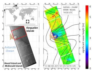
An example of sea state processing under storm conditions with wave height about 3-5 m acquired over the Antarctic Ocean on 05.01.2017. In-situ buoy measurements are not available for this area; the isolines show the wave height from WWIII model of NOAA. The red marked image was proceed in NRT and delivered directly on board the research vessel "Akademik Tryoshnikov".
