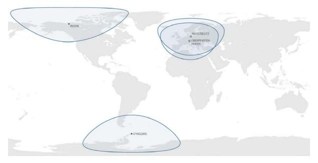
**Fig. 1**. Ground Station Network of the German Remote Sensing Data Center (DFD) of DLR. The blue circles delineate the visibility circles of the receiving stations.
