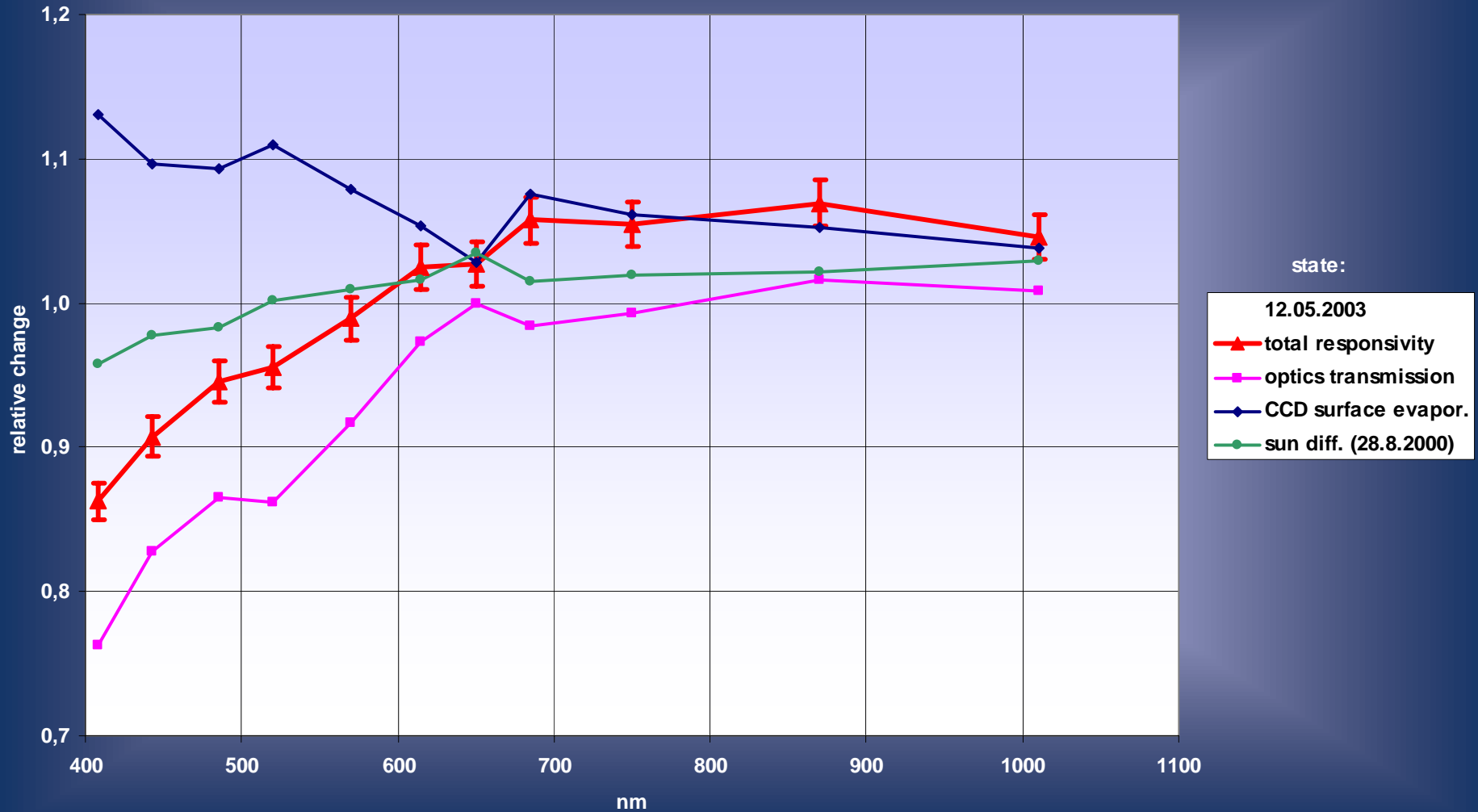
Relative change of MOS - IRS components during mission time
