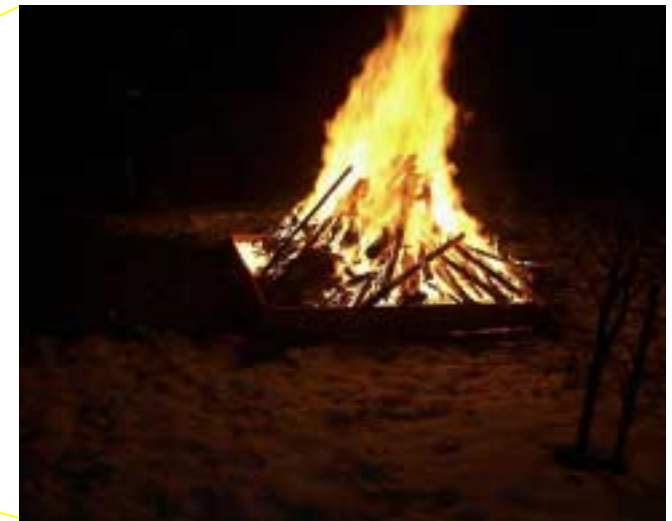
On-ground image of the test fire: Size = 2 \times 2 \text{ m}^2 Max. temperature = 930-990 K Energy release < 0.17-0.22 MW
