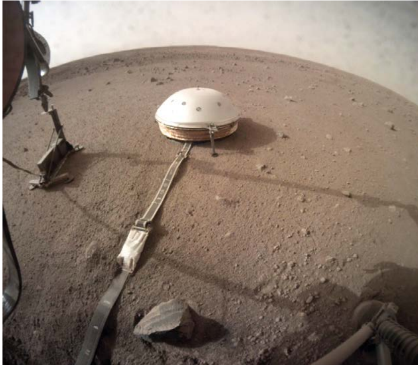
Fig. 5-2 View of InSight camera ICC, deployment of HP 3 on sol 76 (left). SEIS instrument middle. Credit: NASA/JPL-Caltech
