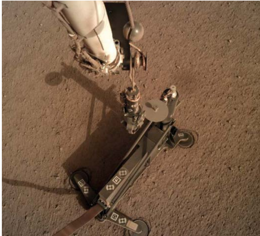
Fig. 5-1 HP 3 after deployment to the Martian surface. InSight deployment arm has released HP 3 . Picture of arm camera IDC. Credit: NASA/JPL-CalTech/DLR
