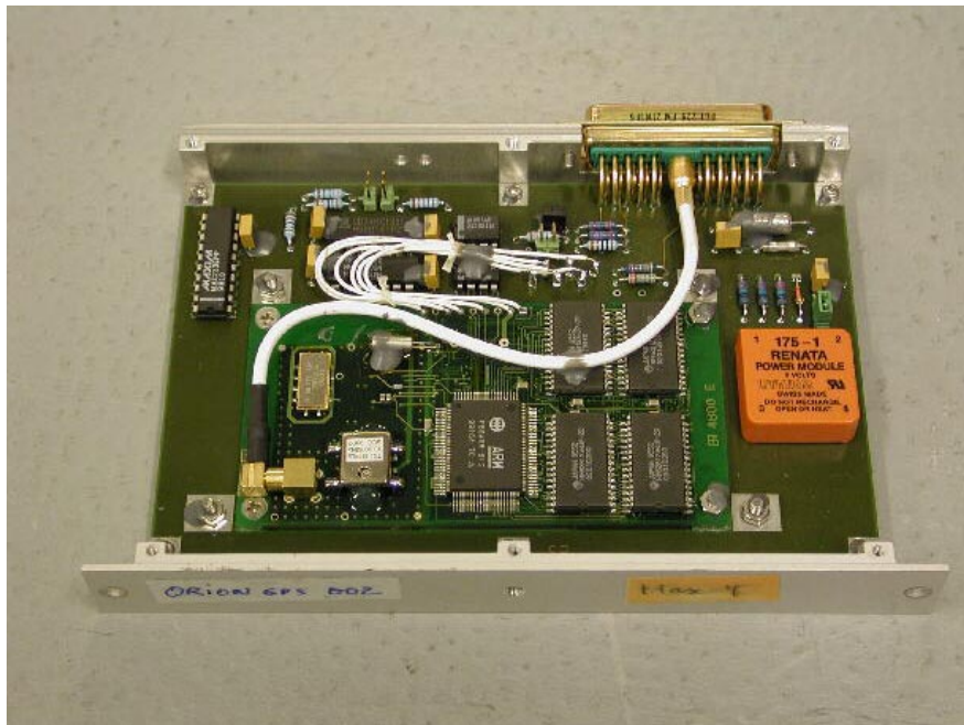
Fig. 1.2 Orion GPS unit for the Maxus-4 flight. The main receiver board is embedded into the KT interface board featuring various serial line drivers and a backup battery. Total outer dimensions are 160 x 110 x 20 mm 3 .
