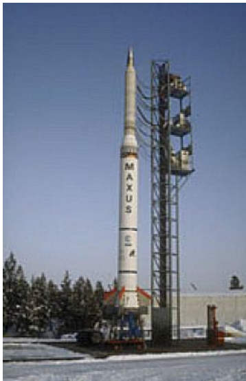
Fig 1.1 The Maxus-4 rocket has an overall length of 17 m. It employs a Castor-4B motor of 10 m size, which is able to carry an 800 kg payload to an altitude of 700 km
