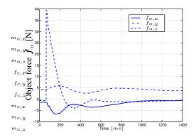
Fig. 11. Object impedance force  $f_0$  during box motion of 4 cm using a translational stiffness of 1000 N/m.
