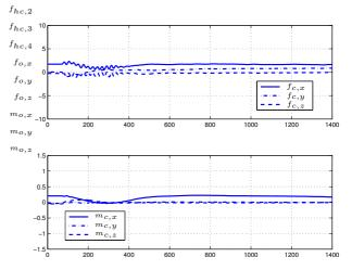
Fig. 13. Spatial coupling impedance force  $m{f}_{c,r}$  and torque  $m{m}_{c,r}$  during box motion of 4 cm. The translational and rotational stiffness were chosen as 500 N/m and 3 Nm/rad, respectively
