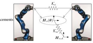
Fig. 3. Two-arm impedance behavior by combining a coupling spring with an object level spring.
