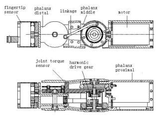
Fig.3: Finger unit with one integrated actuator and two coupled joints.
