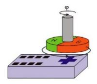
Fig.5: Principle of measuring system by using integrated hall sensor
