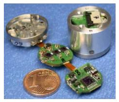
Fig. 6, full digital 6dof fingertip force sensor
