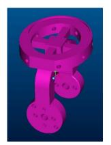
Fig.4: Base joint torque sensor
