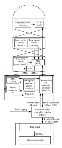
Fig.8: Electronics and communication architecture
