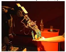
Fig. 8: Tracking and grasping an object.
