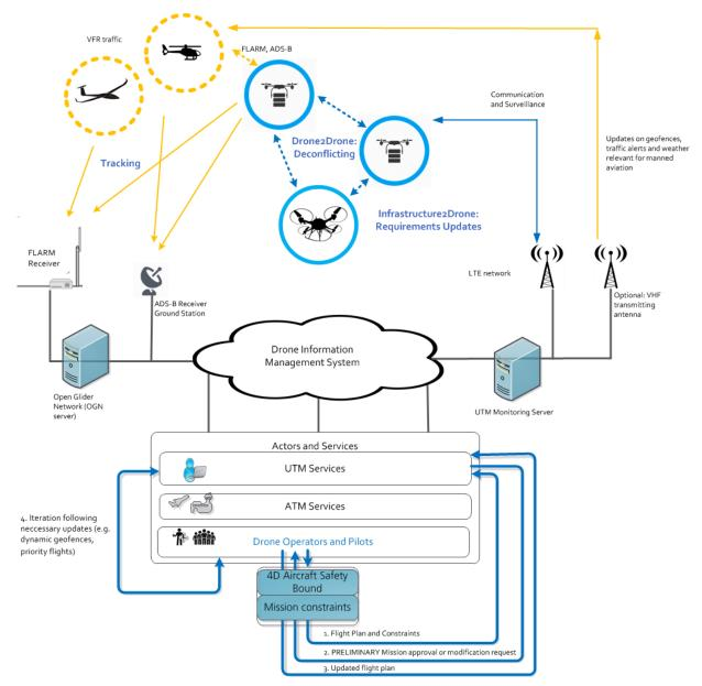
Figure 6: Concept for Communication and Surveillance
