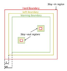
Figure 2: Geofencing Boundaries as introduced by Nasa SAFEGUARD [4]
