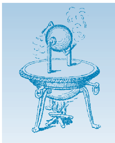
ASME, JT, Jan. 2005. Heron's Aeolipile, a steam-driven rotor (around 60 AD)
