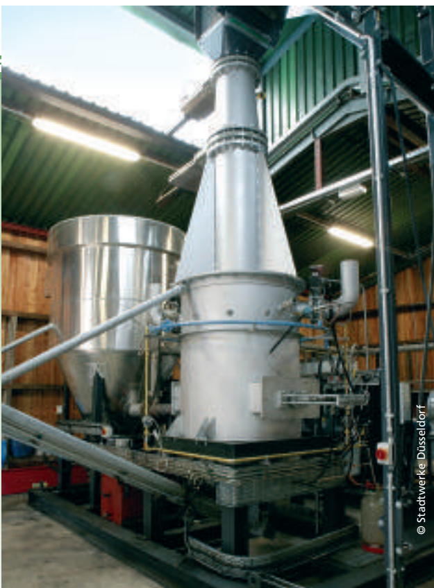
Equipment to extract alternative fuel gases from solid fuels has become an relevant -after treatment technology – a pilot plant for advanced wood gasification set up in Arnsherg by Stadtwerke Düsseldorf, an EnBW holding
