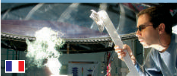
Melting experiment in the 6 kW solar furnace of the PROMES testing plant belonging to the CNRS research group in Odeillo, France (source: CNRS-PROMES)
