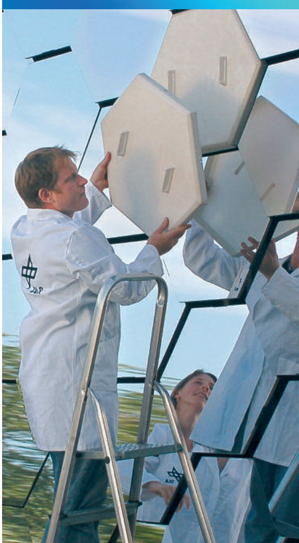
Preparing the solar furnace concentrator for HYDROSOL testing: Jan Peter Säck and Daniela Graf from the DLR Institute of Technical Thermodynamics assemble the mirrors
