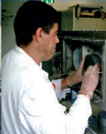
Lamark de Oliveira of the DLR Institute of Technical Thermodynamics assembles the HYDROSOL reactor (EU project HYDROSOL – Catalytic monolith reactor for hydrogen generation from solar water splitting)
