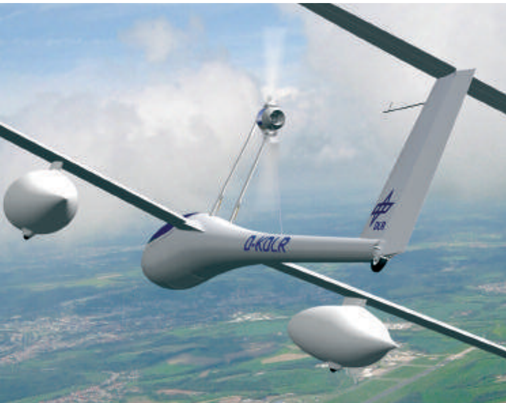
DLR's hydrogen-powered glider with a fuel cell motor – based on the Antares 20E from Lange Aviation
