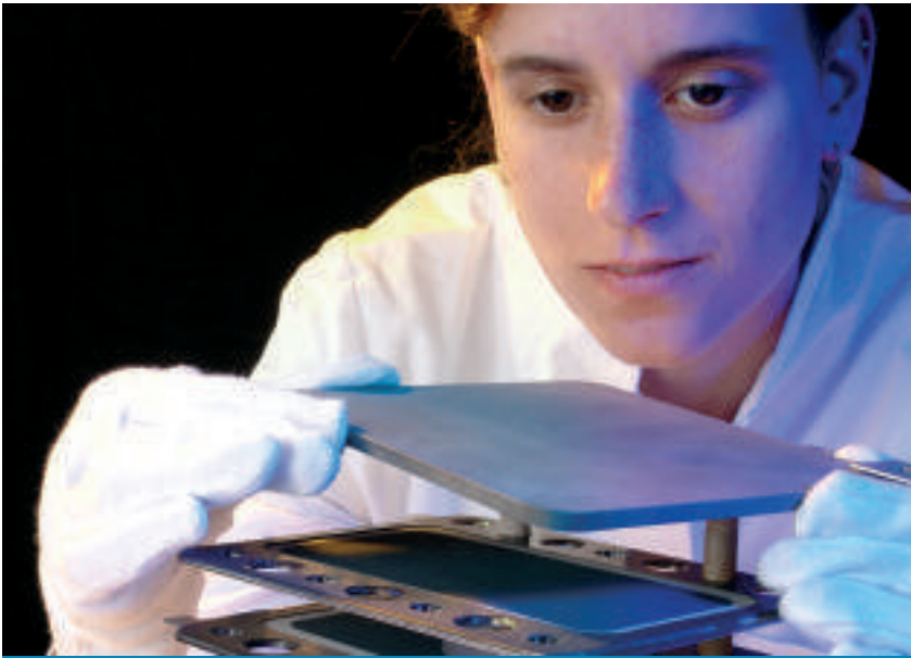
Assembling a high-temperature fuel cell cassette
