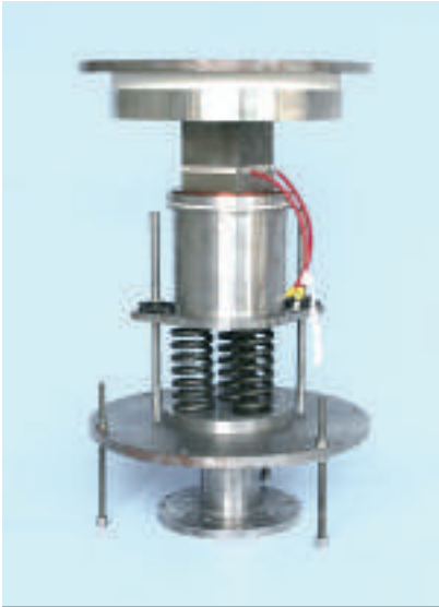
DLR is developing unique measurement technologies for thermoelectric materials and modules. This is the measuring column of a test rig for assessing the efficiency factor and other component properties in real-world conditions.
