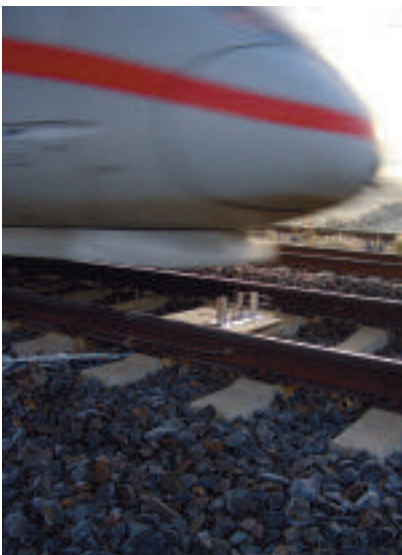
Transit of a high-speed ICE 3 type train over a sensor-equipped panel for determining the speed and pressure field in the undercarriage area of the train.
