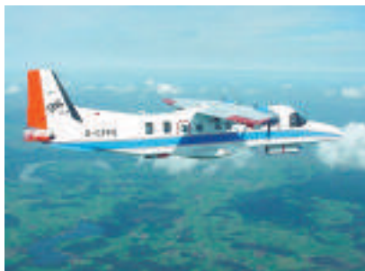
The Dornier Do 228 as a carrier platform for the F-SAR: The antenna system is attached in a radome under the tail of the aircraft.
