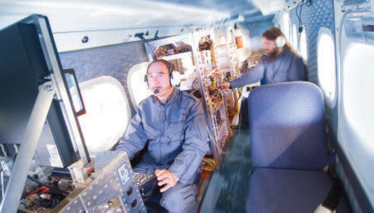
F-SAR radar and operator in action on the Dornier Do 228
