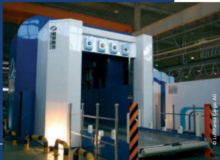
Test facility for the checking of airfreight units
