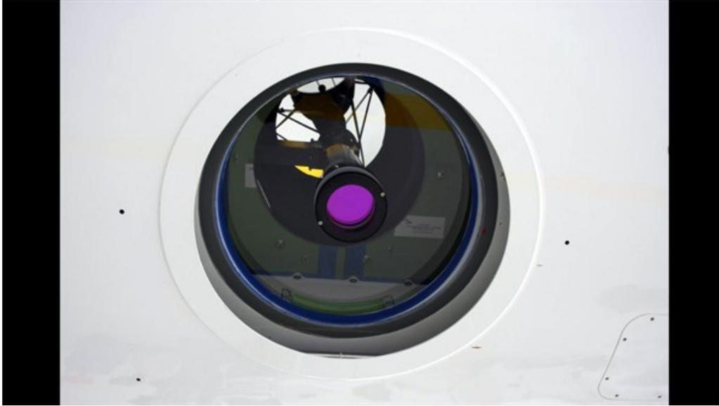
To precisely record the properties of cirrus cloud and vapour trails, the HALO research aircraft is equipped with a lidar system. This image shows the 'optical window', seen from outside the aircraft.
