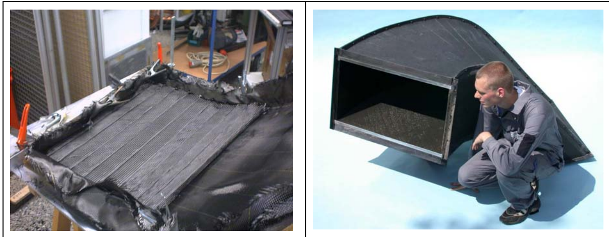
Figure 5: Arrangement of wrapped foam cores (left), final APU Intake Duct (right)
