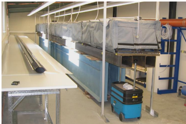
Fig. 6: Production facilities: modular CFRP tooling and bake-out tent for vacuum-bagging and low-cost boom manufacturing.
