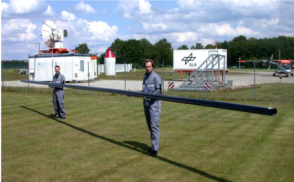
Fig. 1: Deployable CFRP boom. Length 14 m, mass 1.4 kg.
