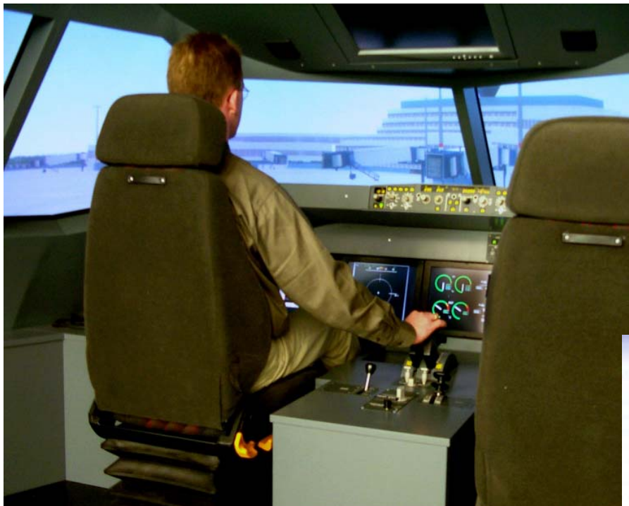
Figure 3: DLR's Cockpit simulator which is equipped with raster capable HUD (HGS 4000 from Flight Dynamics) and head-mounted display (Microvision, retinal scanning device)
