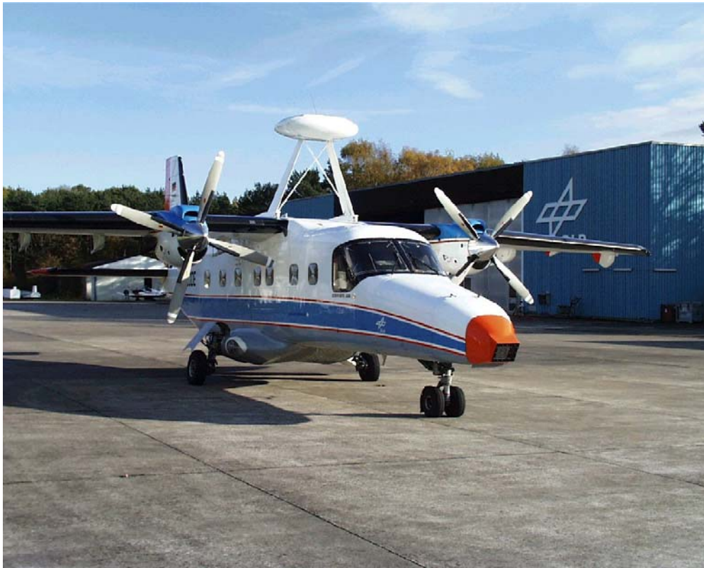
Figure 4: DLR's test aircraft DO-228, equipped with a sensor suite (HiVision MMW radar sensor of EADS, Ulm, Germany, on top, IR-sensor in the nose, DGPS, INS, radar altimeter) and with high performance data recording and data processing systems
