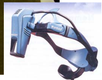
Figure 3: DLR's Cockpit simulator which is equipped with raster capable HUD (HGS 4000 from Flight Dynamics) and head-mounted display (Microvision, retinal scanning device)
