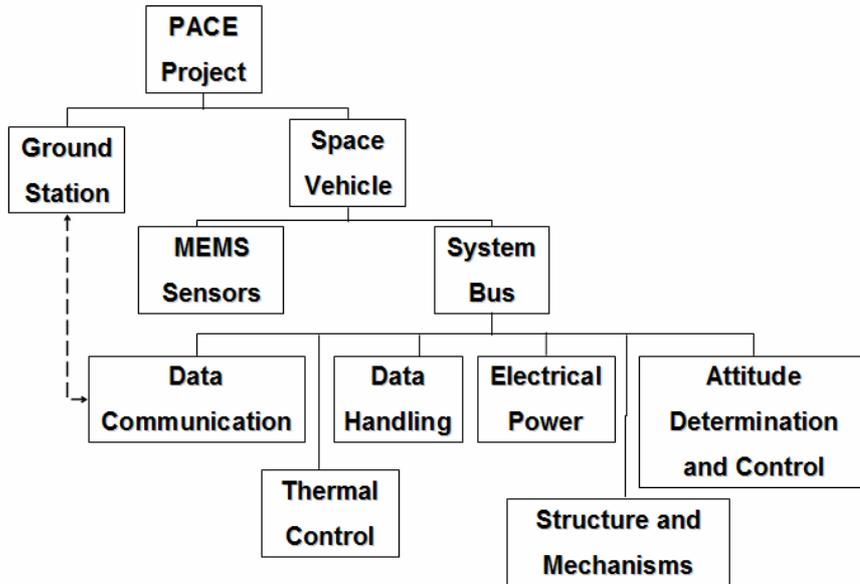
Fig.1 The hierarchy of the PACEsat project
