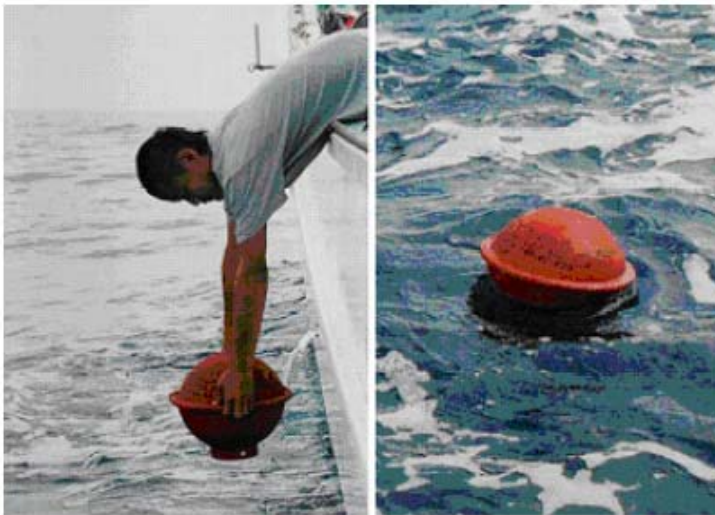
Figure-3 Release and Floating Scene of the Buoy
