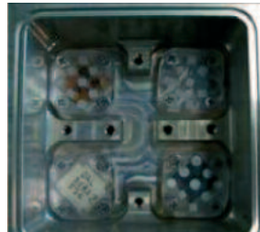
‘Dark control measurement’ positions at the bottom of the experimental container of EXPOSE
