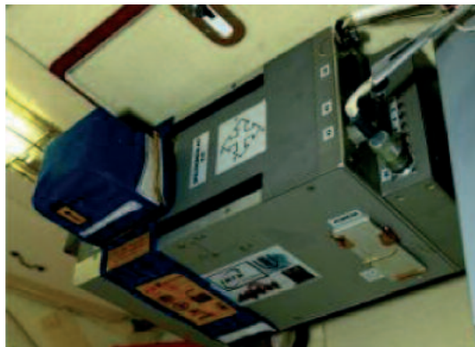
ALTEINO with the shielding tile experiment (passive detectors from DLR)
