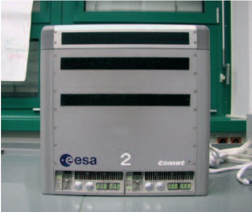
KUBIK is a mobile ESA incubator facility for cell biological research that is used during the Soyuz missions to ISS
