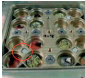
‘Depth dose measurement’ positions at the top of the experimental container of EXPOSE (red circle)
