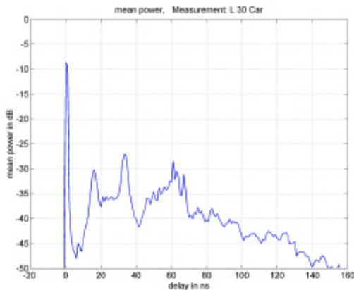
Figure 20: Mean expected power, urban 30° elevation
