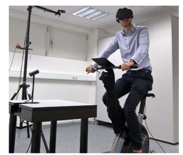
Fig. 1: Experimental setup with bike ergometer and HMD.
