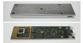
Fig. 3: The prototype of the DLR developed M-42 active radiation detector.
