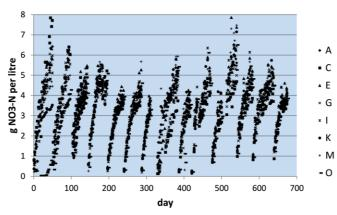
Fig. 3: Fed batch. Nitrate production of eight filters, which were fed with 1 l of synthetic urine per day over a period of 680 days.
