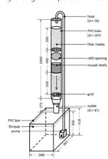
Fig. 1: The C.R.O.P.® filter. The liquid flow is cyclic. The filtrate passes repeatedly through the filter, until the process is finished. Internal dimensions are given in mm.
