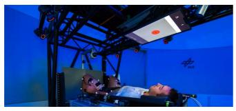
Fig. 2: Subject position on the jumping sledge at the DLR-SAHC during the JUMP-study.
