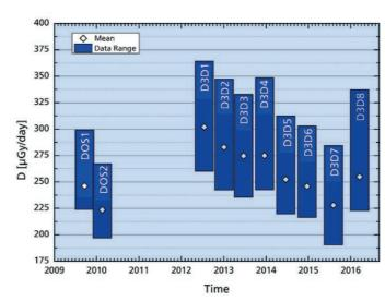
Fig. 1: Variation of the absorbed dose measured with passive radiation detectors inside Columbus for 2009-2017 [1.2].
