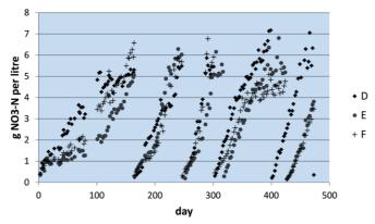
Fig. 2: Batch mode. Nitrate production of the filters D,E,F, which were fed with batches of 80% urine solution over a period of 475 days.
