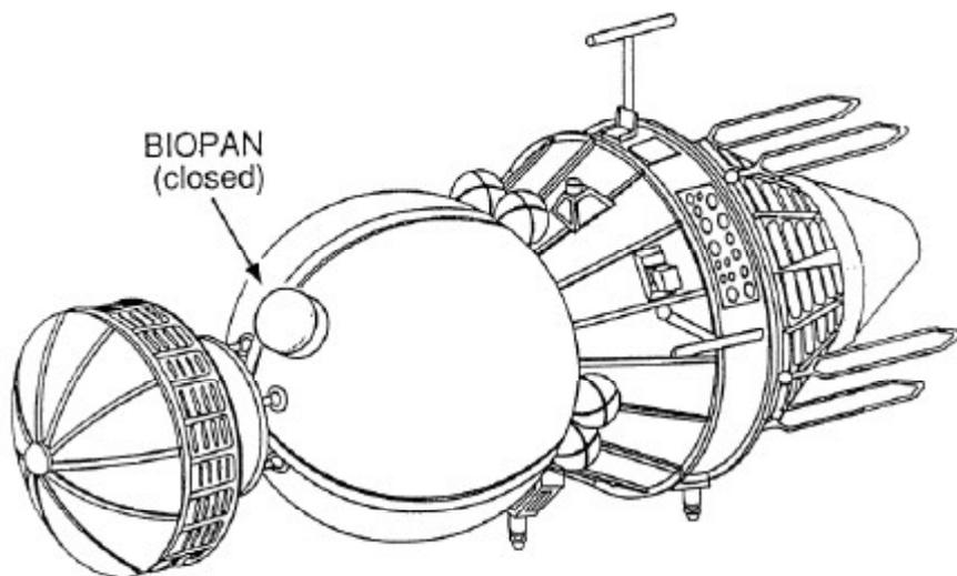
**Fig. 15.6** The exposure facility BIOPAN mounted on the satellite.
