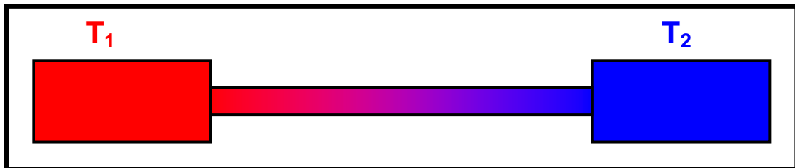
Soret effect Co in Sn, T_0 = 500 \text{ }^\circ\text{C}
