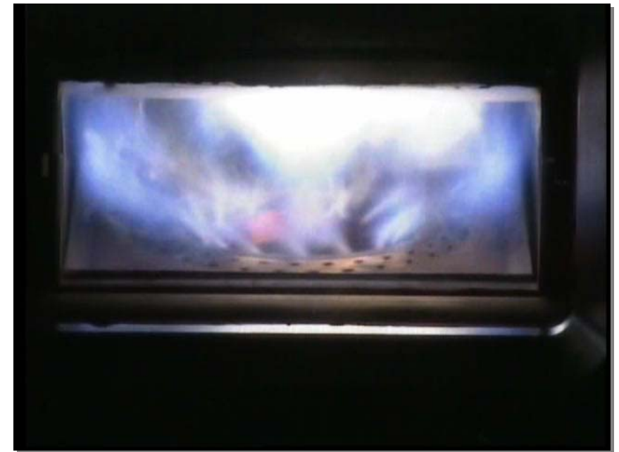
DLR Investigation of RR-D lean burner module with internal staging
