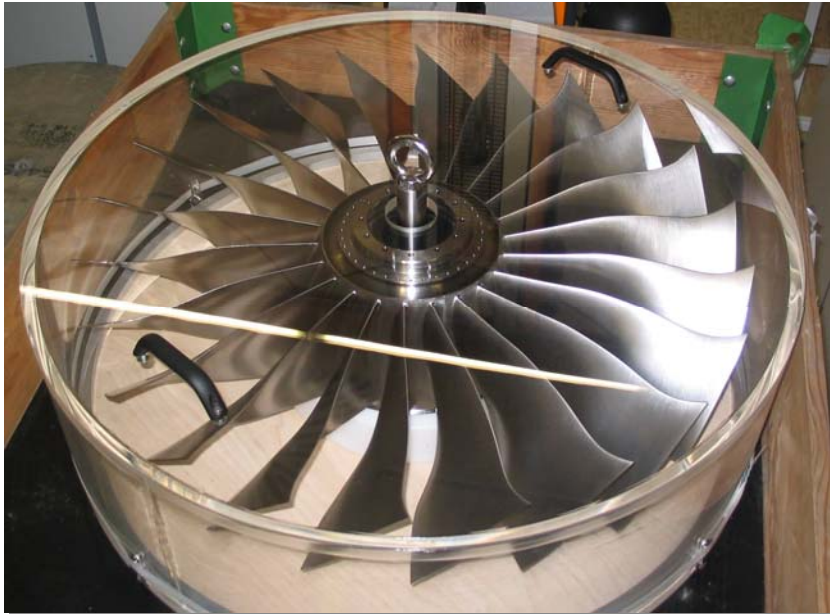
Geared Fan (BPR = 12) Tests at DLR starting in 2007
