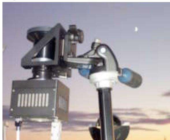
Fig. 1: SPOSH breadboard at dusk, ready for meteor observations
