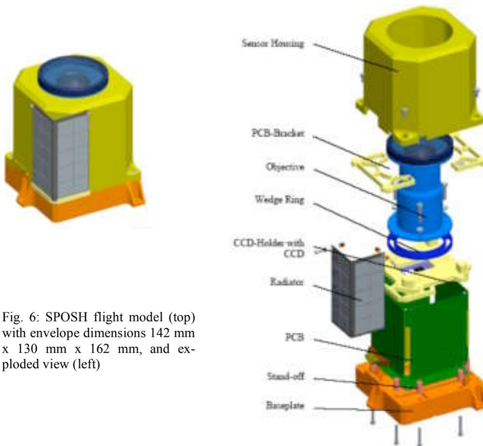
Fig. 6: SPOSH flight model (top) with envelope dimensions 142 mm x 130 mm x 162 mm, and exploded view (left)
