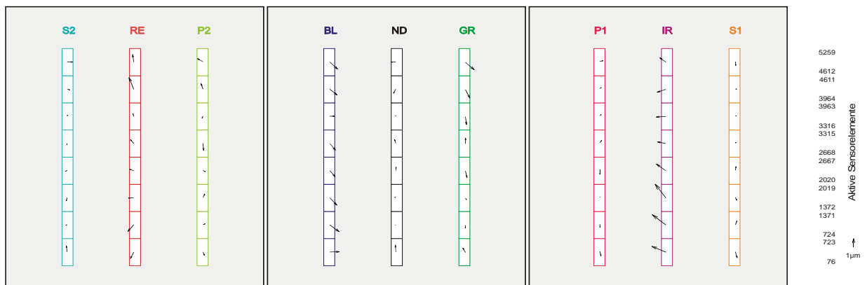
Figure 4: Systematic residuals at the image coordinates (orbit 2063) after adjustment of interior orientation. Each of the 9 lines is divided in 8 parts. For these parts the root mean square error is showed.
