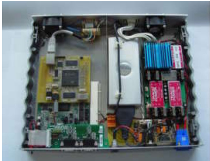
SPS Electronic Box with DPU, Camera head interface and Power supply
