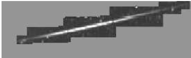
Fig. 5: Slow-moving (approx. 33 km/s) Geminid detected on 8 consecutive images, extending over more than 50 pixels. The camera operated at a frame rate of 2 frames per second. The Figure shows the windows of interest returned by the camera processor
