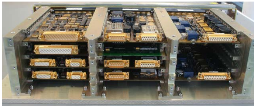
Fig. 9. Testing of the payload supply system in a test rack
